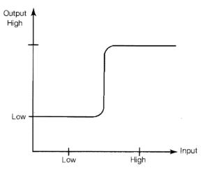
Fig. 1. The typical nonlinearity for an analog implementation of a digital design.
