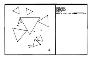
This demonstration shows our general approach to object recognition as applied to the simplified domain of equilateral triangle recognition. The input to the system is the collection of vertices of a set of non-overlapping equilateral triangles whose size, location, and orientation are chosen randomly. A control specifies the number of triangles in the input. The goal of the system is to parse this set of vertices into equilateral triangles.
